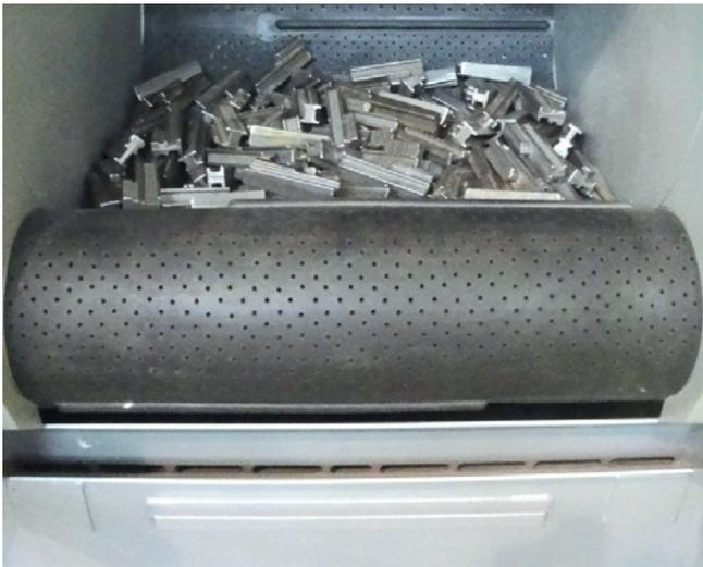
GRITROLL belts are used on Shot and Sand-blasting machines, usually for finishing small parts loaded in bulk and, in its cradle-configuration, it gets the parts to be worked and keep them in continuous tumble.
