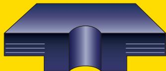
Transfer belts often have a guide on the bottom of the belt to keep the drainage holes centered over the vacuum chamber and to aid in tracking. In some cases multiple guides are found on the bottom of the belt for increased capacity. Drain holes run through the transfer belt and bottom guide when the guide is located over the vacuum channel.
